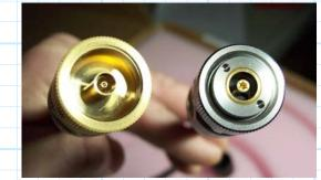
The top of the line connector. Best performance, but cost **big \$\$\$**. Used primarily in test equipment (e.g., network analyzers). 3.5 can work to nearly 40 GHz.
