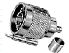
The **original** microwave connector. Good performance (up to 18GHz), and moderate cost, but large (about 2 cm in diameter)! However, can handle greater **power** than SMA.
